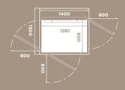
Size:  $900 \times 1280 \text{ mm}$  Rated load: 410 kg
